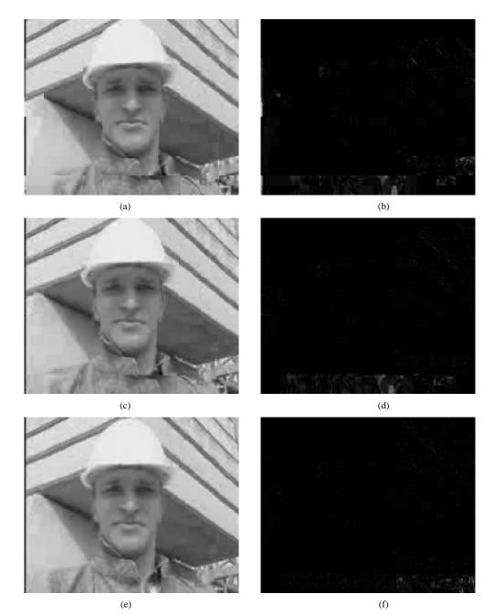
Fig. 7. Illustrations of error-recovery effects. (a) Frame 1 of the Foreman sequence, error condition C9. The error is large because the error packet in the I frame is resent and the bandwidth loss is accumulated into Frame 1. (b) Error frame of frame 1. (c) Frame 2 of the Foreman sequence. (d) Error frame of frame 2, error is less than frame 1. (e) Frame 3 of the Foreman sequence. (f) Error frame of frame 3. More errors are recovered and new errors are generated at the bottom-right MBs.
