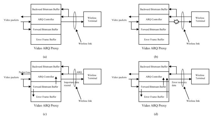
Fig. 4. Illustration of video ARQ proxy behavior. (a) Normal condition. (b) An error occurs on the wireless link. (c) Important data resent and texture residual decoded into error-frame buffer. (d) Recovery of texture errors.
