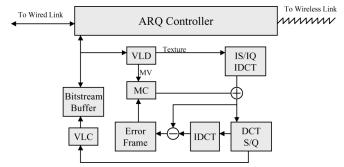
Fig. 5. Block diagram of video ARQ proxy server.
