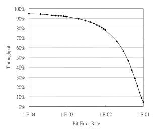
Fig. 10. Maximum throughput using BCH code under various error conditions. Packet length =511 bits.
