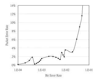
Fig. 11. Packet error using BCH under various error conditions when maximum throughput is achieved. Packet length =511 bits.
