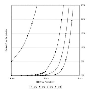
Fig. 8. Packet error under various error conditions and error-correction codes. Packet length = 511 bit.
